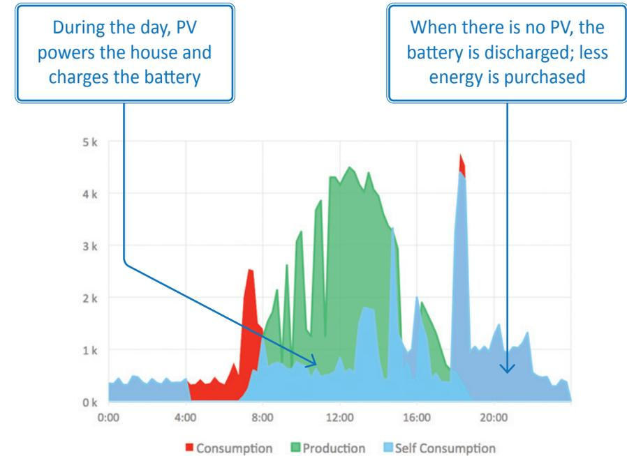
\* Based on a SolarEdge 5kW PV system installed on a residence in Germany
