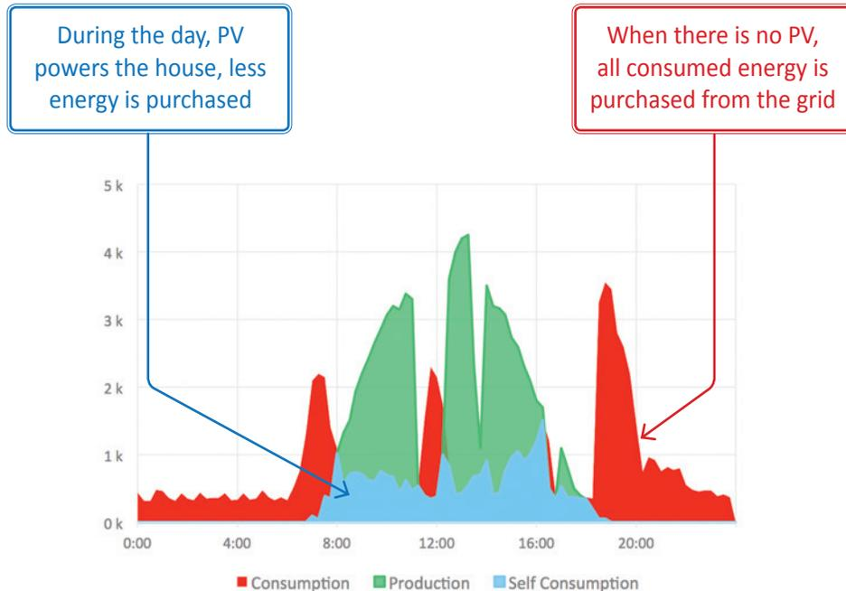
\* Based on a SolarEdge 5kW PV system installed on a residence in Germany
