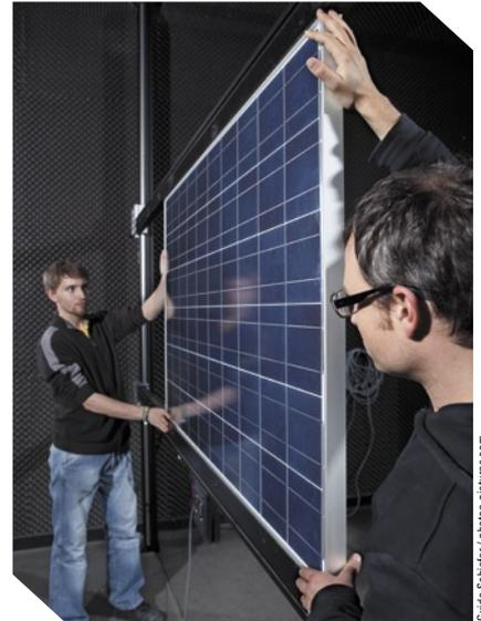
**PHOTON Lab measured the weak-light behavior of modules in its sun simulator.**
